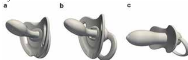
3D complete models of the tested pacifiers: a. Orthodontic Pacifier; b. Standard Pacifier; c. Conventional Pacifier.
