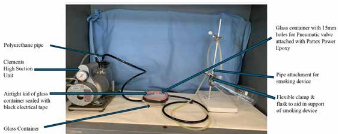
Figure 1: Set up of machine which mimics smoking
