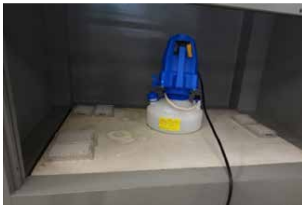
Image 3: Portable electric ULV cold vaporiser in ventilated fume cupboard
